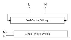
For Dual-Ended Lamps, the pins on each end of the lamp are internally shunted. The lamps may be used with shunted or un-shunted tombstones.
