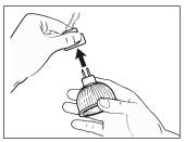
1. Align the GU10/GU5.3 pins of MR16 with the base holes
