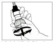
2. Push the MR16 bulb into the base and rotate clockwise to lock it.
