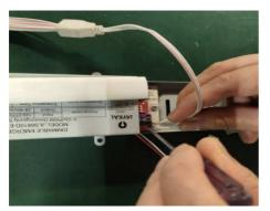
Step 3. Connect the AC wires
