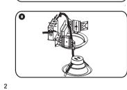
Step 9: Wire nut the ground (green) wire in the junction box. Wire nut the black input wire with the black wire from the MC cable and wire nut the white input wire with the white wire from the MC cable. Wire nut the purple input wire with the purple wire from the MC cable and wire nut the pink input wire with the pink wire from the MC cable. If the purple and pink wires are not in use, cap these wires individually with wire nuts.
