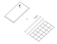
3. Mechanically secure the led driver in original troffer wiring compartment
