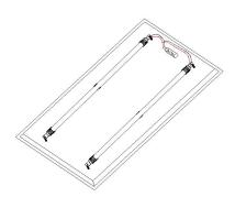
4-5. In order to get more security to don't make the led strips fall down few years later, can drill two screws( self drilling screw) through screw holes of strips into the bottom of troffer.
