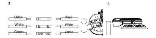
Connect the input AC cable from fixture with cable from power supply by connecting with same color wire, black for L, White fro N, Green for Ground
