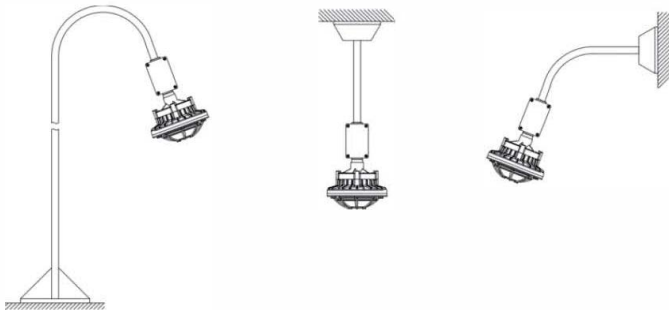
Figure 4 Pole Mount (With junction box)
