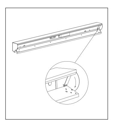
4.Install anchoring bolt.Drill four holes in the corresponding position on the wall according to the positioning plate provided by the manufacturer. Insert an anchoring bolt (not included) into each hole.
