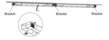
4.Fix the safety cables to the original housing. Hang the LED retrofit assembly with the cables and make electrical connections. Secure the assembly with fixing clips.
