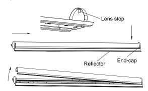
5.Depress and insert the lens past the lens stop inside the end-cap. Snap the lens upward into the reflector track. Carefully slide lens and make sure both ends of the lens are completely wrapped by end-caps. Check and make sure the end-cap perpendicular to the reflector.
