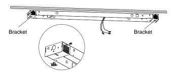
4.Fix the safety cables to the original housing. Hang the LED retrofit assembly with the cables and make electrical connections. Secure the assembly with fixing clips.
