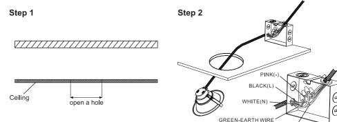
Cut hole in ceiling according to cutout template for each model
