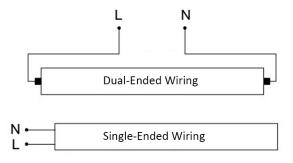
For Dual-Ended Lamps, the pins on each end of the lamp are internally shunted. The lamps may be used with shunted or un-shunted tombstones.
