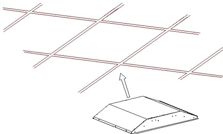
**Step 1:** Pass the troffer through the opening of the ceiling (T-grid).
