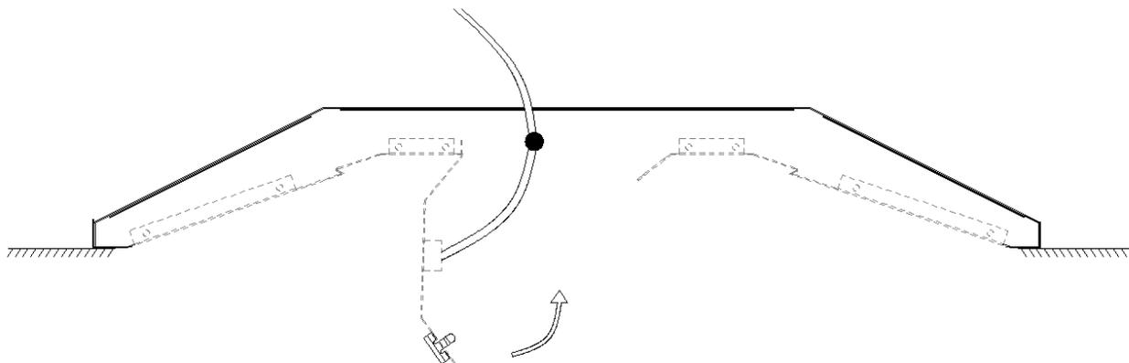
Complete the AC wiring connection between troffer LED driver and the AC supply lines.
