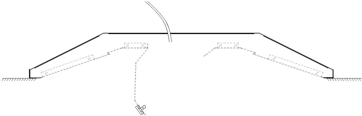
Set the troffer into the grid. Inspect the fit of the troffer in the grid. The troffer should be lying flat in the grid with no gaps. Open the wiring cover using the twist locks. Pass the AC supply lines through the hole on top of the troffer housing or the side of the housing, depending upon the application.
