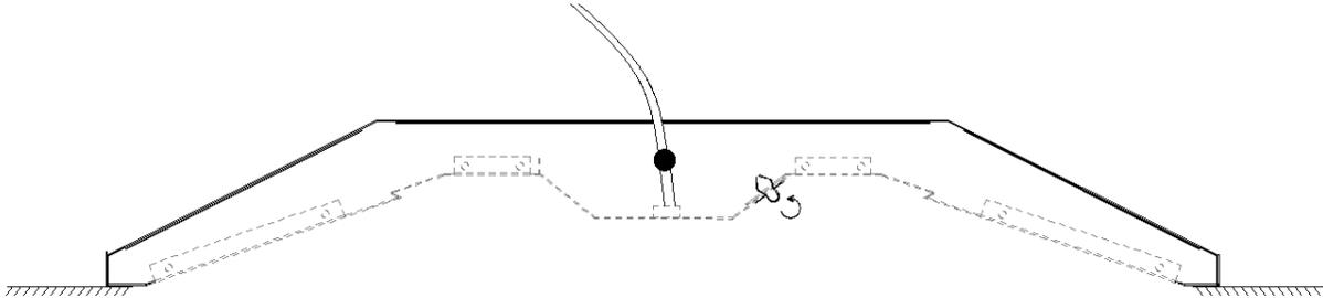
Return the wiring cover to the closed position and use the twist locks to secure the cover
